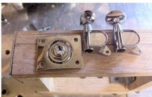
12. Use eight small eye screws to guide the strings off of the cabinet handle to the tuners. The four eye screws in the middle should be spaced to the desired string spacing. The eye screws on the sides should be placed so that they are in line with the guitar tuners. If amplification is being used, place the two eye screws on the side of the jack plate so they miss the audio jack.
