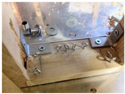
13. On the top of the box, two metal corner braces will be mounted with the small bolts through the wood to the metal braces on the inside of the box. The braces on the top of the box will form a channel to mount the neck. If desired, have one of the bolts longer so that a strap peg can be mounted on top of the bracket. The other strap peg will be in the middle of the wood on the back bottom of the box.
