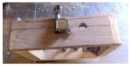
11. If amplification is desired, drill out a hole for the mono audio jack and square jack plate.
