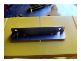
10. Drill four holes for the desired guitar style tuners. Mount the tuners as close to the front of the box as possible.
